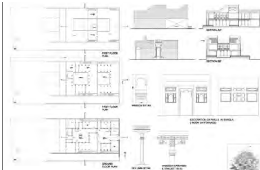
Figure 8: Documentation of one Wada changing its face and now major part of it is in dilapidated condition (Red dotted line is part of Wada which is in damaged condition), made by Vaidehi Lavand (Dotted line, appearing in the Plans on the left figure appearing in the elevation on right figure, is a part of Wada which is in damaged condition.)
